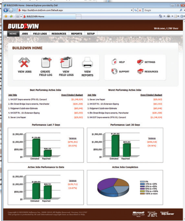
Figure 2 – The BUILD2WIN home page includes a customizable digital dashboard which allows you to drill down to any level of job performance detail on-screen.
